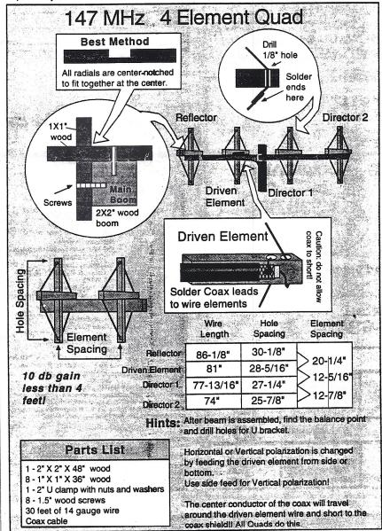
Cut four pieces of wire about 6 inches longer than the measurements shown. Feed each wire through the four holes in the cross elements. Twist together the ends and solder the joint.
